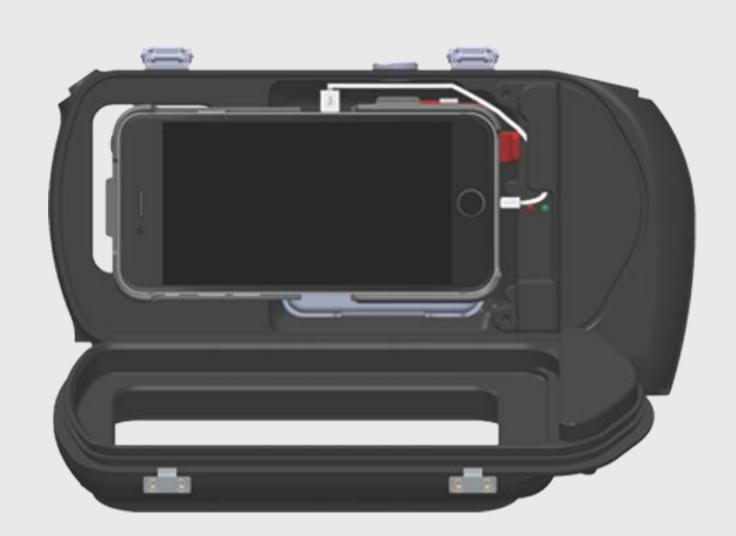
4. Press the power switch. The red LED will start flashing, and the Smartphone screen will turn on (being under charge).
